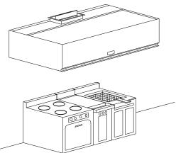
eliminates cold drafts, and hot spots, enhances the capture capability of the filter hood and results in a more comfortable kitchen environment. A supply air volume up to 80% of the total exhaust is recommended. The fresh air should be tempered to between 55 and 75F (13 to 24C)
