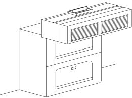
satisfactory for oven applications. Directing the make up air through the front of the hood provides the correct air quantity and excellent distribution within the kitchen..
