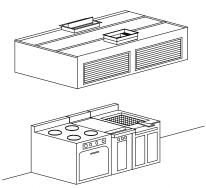
The total exhaust to properly ventilate commercial kitchen is directly related to the type of cooking equipment under the filter hood. An exhaust flow rate of between 150 to 400 CFM/ft. (233 to 620 l/s/m) is satisfactory for most installations. Directing the make-up air through the front of the hood provides the correct air quantity and excellent distribution within the kitchen
