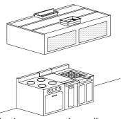
The total exhaust to properly ventilate commercial kitchen is directly related to the type of cooking equipment under the filter hood. An exhaust flow rate of between 150 to 400 CFM/ft. (233 to 620 l/s/m) is satisfactory for most installations. Directing the make-up air through the front of the hood provides the correct air quantity and excellent distribution within the
