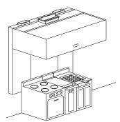
flow rate between 150 and 400 CFM/ft (233 and 620 l/s/m) is satisfactory for most applications. Introducing supply air back into the kitchen is good engineering practice. An adequate supply of fresh air eliminates cold drafts, and hot spots, enhances the capture capability of the filter hood and results in a more comfortable kitchen environment. A supply air volume up to 60% of the total exhaust is recommended. The fresh air should be tempered to between 45 and 75F (13 to 24C)
