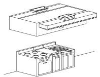
The total exhaust to properly ventilate commercial kitchen is directly related to the type of cooking equipment under the filter hood. An exhaust flow rate of between 150 to 400 CFM/ft (233 to 620 l/s/m) is satisfactory for most installations. Directing the make up air down, from the front of the hood provides continuous air movement, directed towards the cook.
