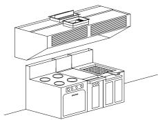
equipment under the filter hood. An exhaust flow rate of between 150 to 400 CFM/ft. (233 to 620 l/s/m) is satisfactory for most installations. Directing the make-up air through the front of the hood provides the correct air quantity and excellent distribution within the kitchen.
