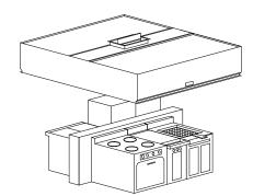
The total exhaust required to properly ventilate a commercial kitchen is directly related to the type of cooking equipment under the ventilator. An exhaust flow rate between 300 and 700 CFM/ft (465 and 1085 l/s/m) is satisfactory for most applications. For detailed calculations refer to the *Spring Air Systems Ventilator Engineering Manual*.
