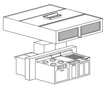
flow rate between 300 and 700 CFM/ft (465 and 1085 l/s/m) is required for most hoods. Heated fresh air is discharged out the front of the hood canopy for MP and MG types. Fresh air volume of 80% of the total exhaust is recommended for heated makeup air systems. Refer to the *Ventilator Engineering Manual* for supply air volume calculations.
