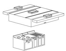
under the ventilator. An exhaust flow rate between 200 and 600 CFM/ft (310 and 930 l/s/m) is required for most hoods. Refer to the *Ventilator Engineering Manual* for supply air volume calculations.
