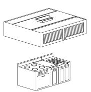
700 CFM/ft (465 and 1085 l/s/m) is required for most hoods. Heated fresh air is discharged out the front of the hood canopy for MP and MG types. Fresh air volume of 80% of the total exhaust is recommended for heated makeup air systems. Refer to the Ventilator Engineering Manual for supply air volume calculations.
