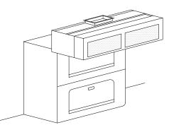
between 100 and 150 CFM/ft (155 and 2331/s/m) is satisfactory for oven applications. Directing the makeup air through the front of the hood provides the correct air quantity and excellent distribution within the kitchen..
