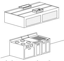
The total exhaust to properly ventilate commercial kitchen is directly related to the type of cooking equipment under the filter hood. An exhaust flow rate of between 150 to 400 CFM/ft. (233 to 620 l/s/m) is satisfactory for most installations. Directing the make-up air through the front of the hood provides the correct air quantity and excellent distribution within the kitchen. .
