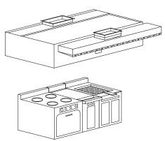
The total exhaust to properly ventilate commercial kitchen is directly related to the type of cooking equipment under the filter hood. An exhaust flow rate of between 150 to 400 CFM/ft (233 to 620 l/s/m) is satisfactory for most installations. Directing the make up air down, from the front of the hood provides continuous air movement, directed towards the cook.
