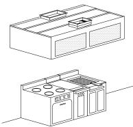
equipment under the filter hood. An exhaust flow rate of between 150 to 400 CFM/ft. (233 to 620 l/s/m) is satisfactory for most installations. Directing the make-up air through the front of the hood provides the correct air quantity and excellent distribution within the kitchen.
