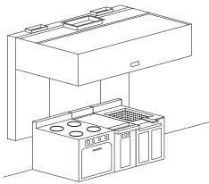
Introducing supply air back into the kitchen is good engineering practice. An adequate supply of fresh air eliminates cold drafts, and hot spots, enhances the capture capability of the filter hood and results in a more comfortable kitchen environment. A supply air volume up to 60% of the total exhaust is recommended. The fresh air should be tempered to between 45 and 75F (13 to 24C)
