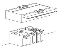
The total exhaust to properly ventilate commercial kitchen is directly related to the type of cooking equipment under the filter hood. An exhaust flow rate of between 150 to 400 CFM/ft (233 to 620 l/s/m) is satisfactory for most installations. Directing the make up air down, from the front of the hood provides continuous air movement, directed towards the cook.
