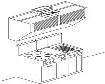
equipment under the filter hood. An exhaust flow rate of between 150 to 400 CFM/ft. (233 to 620 l/s/m) is satisfactory for most installations. Directing the make-up air through the front of the hood provides the correct air quantity and excellent distribution within the kitchen.
