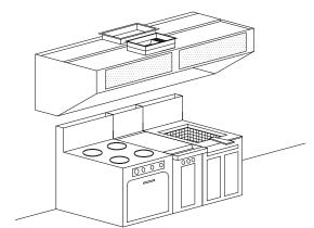
equipment under the filter hood. An exhaust flow rate of between 150 to 400 CFM/ft. (233 to 620 l/s/m) is satisfactory for most installations. Directing the make-up air through the front of the hood provides the correct air quantity and excellent distribution within the kitchen.
