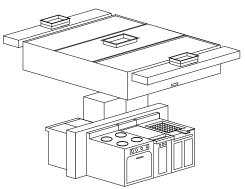
The total exhaust required to properly ventilate a commercial kitchen is directly related to the type of cooking equipment under the ventilator. An exhaust flow rate between 300 and 700 CFM/ft (465 and 1085 l/s/m) is required for most hoods. Heated fresh air is discharged out the front of the hood canopy for MP and MG types. Fresh air volume of 80% of the total exhaust is recommended for heated makeup air systems.
