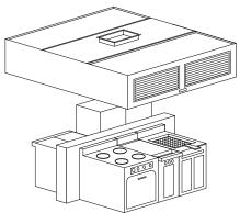
l/s/m) is required for most hoods. Heated fresh air is discharged out the front of the hood canopy for MP and MG types. Fresh air volume of 80% of the total exhaust is recommended for heated makeup air systems. Refer to the *Ventilator Engineering Manual* for supply air volume calculations.
