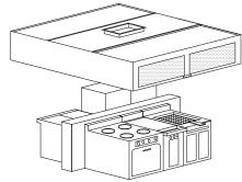
flow rate between 300 and 700 CFM/ft (465 and 1085 l/s/m) is required for most hoods. Heated fresh air is discharged out the front of the hood canopy for MP and MG types. Fresh air volume of 80% of the total exhaust is recommended for heated makeup air systems. Refer to the *Ventilator Engineering Manual* for supply air volume calculations.
