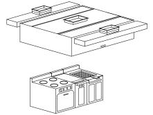
under the ventilator. An exhaust flow rate between 200 and 600 CFM/ft (310 and 930 l/s/m) is required for most hoods. Refer to the *Ventilator Engineering Manual* for supply air volume calculations.
