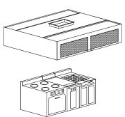
flow rate between 300 and 700 CFM/ft (465 and 1085 l/s/m) is required for most hoods. Heated fresh air is discharged out the front of the hood canopy for MP and MG types. Fresh air volume of 80% of the total exhaust is recommended for heated makeup air systems. Refer to the *Ventilator Engineering Manual* for supply air volume calculations.
